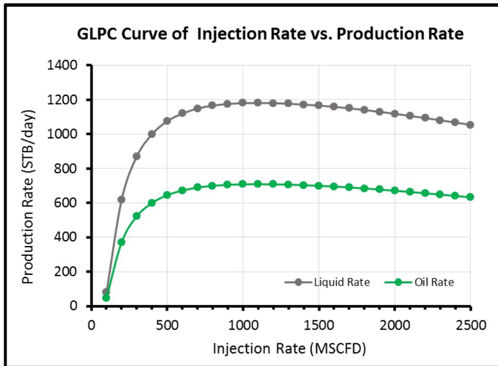
Figure 5. GLPC of Injection Rate against Production Rate
