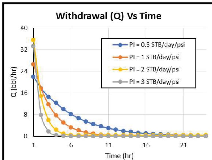
Figure 2. Plot of Withdrawal Rate to Evaluate Equalized Time
