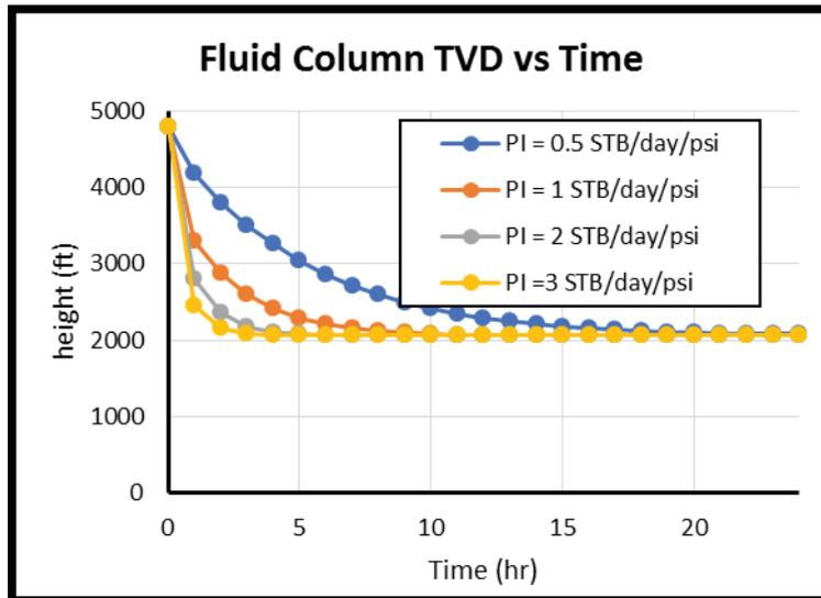
Figure 3. Plot of Killing Fluid Depth to Evaluate Equalized Time
