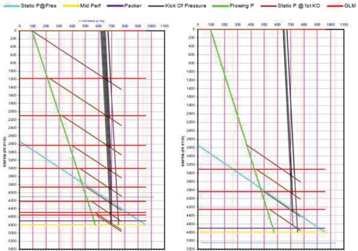
Figure 4. Comparison between Gas Lift Spacing Design Flow Diagram of Conventional Method (left) and Equalized Method (right)
