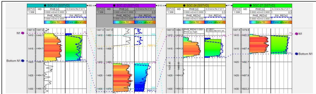
Fig. 7- Sw Model Validation of Capillary Pressure Reconstruction from Petrophysical Log
