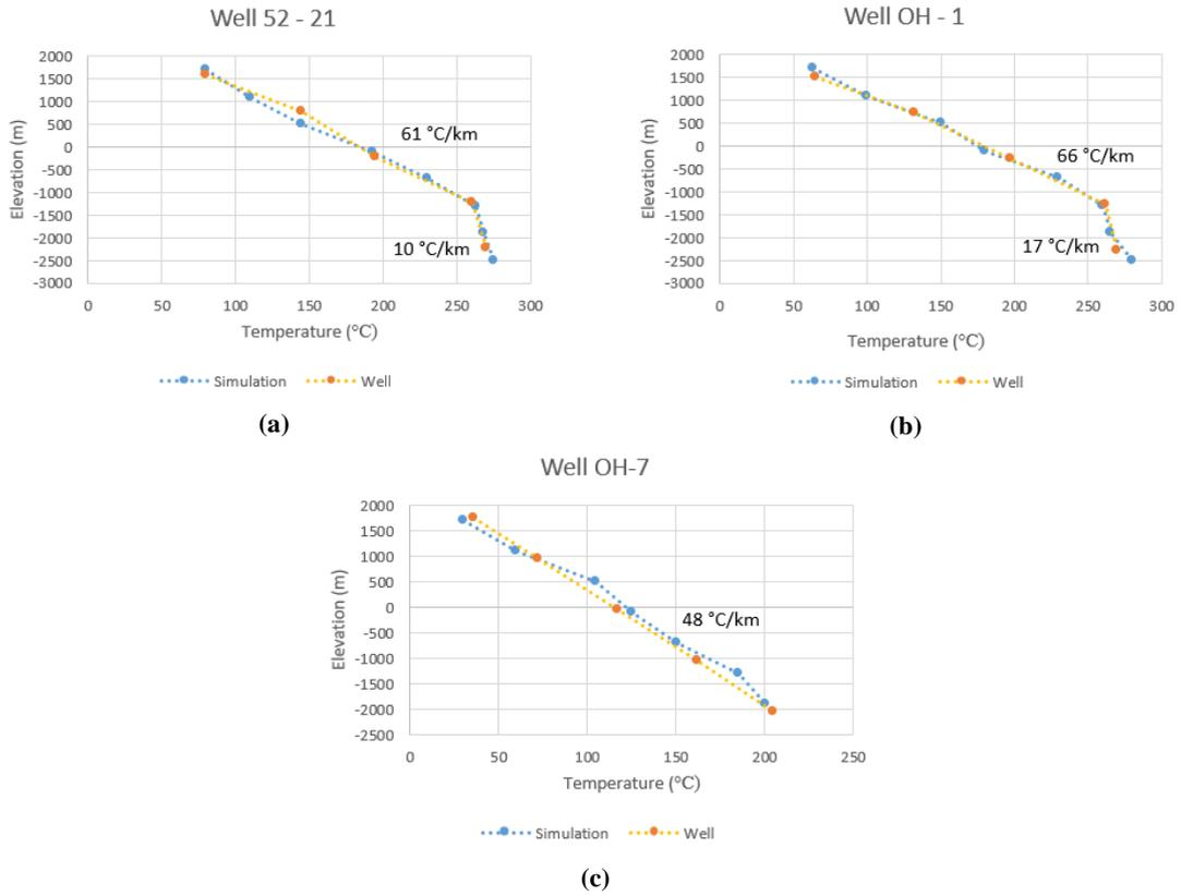
Figure 3: Curve matching for well 52-21 (a), OH-1 (b), and OH-7 (c). Blue dots represent the simulated temperature values while orange dots represent the values from well data. The temperature gradients for each curve are shown near the curve.
