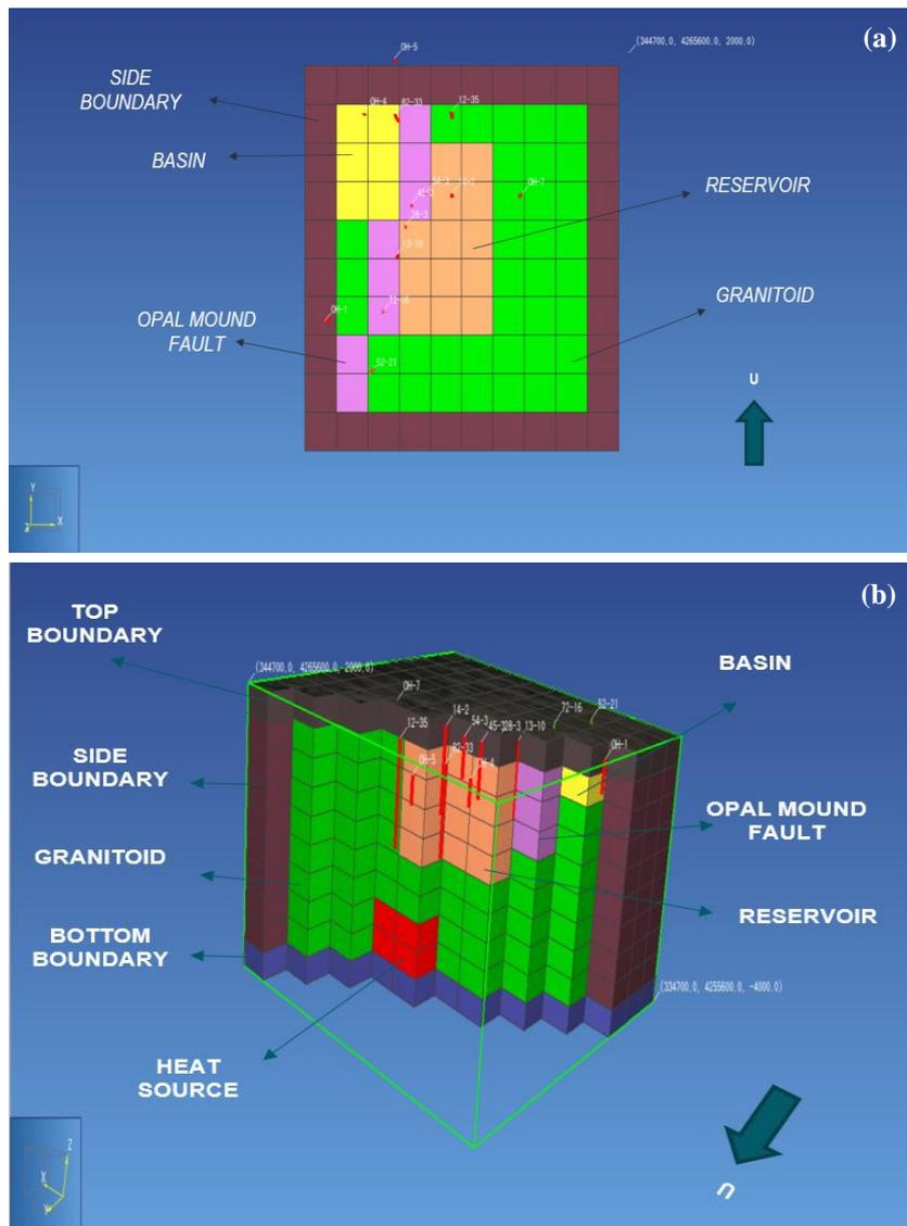
Figure 1: Map view (a) and cross section (b) of the RHS geothermal system simulation model. The model is made based on Simmons et al. (2018) conceptual model with production, injection, exploration, and monitoring wells located in the study area.
