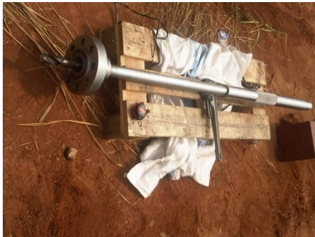
Figure 6 Setting D-904 Drilling Machine, Complete with Twist Drill
