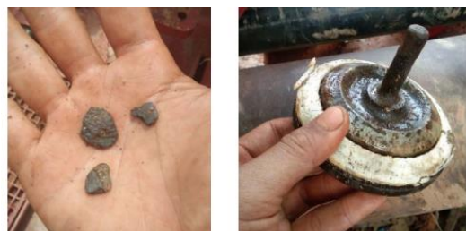
Figure 16 Investigation Result Showed Improper Suction Frac Valve Condition due to Unwanted Pumped Solid Material
