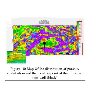
The location of the new proposed well point is depicted with a small black circle symbol on the map. If viewed from the point of the location, it is around the seismic cross-section on inline 1495 and xline 5830.
