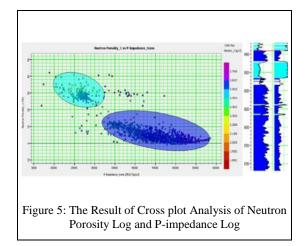
The circled zone in light blue is a target zone with an Acoustic Impedance value of around 24,000((ft/s)\*(g/cc)) - 32,000((ft/s)\*(g/cc)) that has a high neutron porosity of 22% - 44%. While the dark blue circled zone is a bad reservoir zone in the range of acoustic impedance values >33,000((ft/s\*(g/cc))) which has a range of neutron porosity values <15%.
