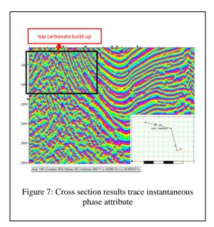
The area in the black box is the result of extraction of the attributes of the targeted research area so that it will make it easier to find the top build up carbonate. The inversion process is carried out on the top tuban of the carbonate reservoir.
