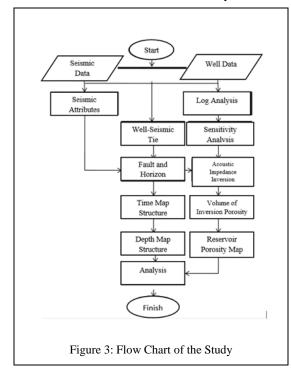
Seismic attributes and acoustic impedance inversions are used to analyze physical lithology and the presence of reservoir hydrocarbon fluids.
