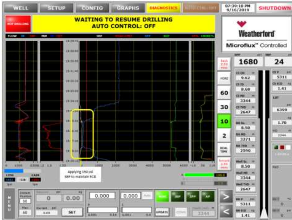
Figure 4: Applying SBP during Connection to maintain ECD.
