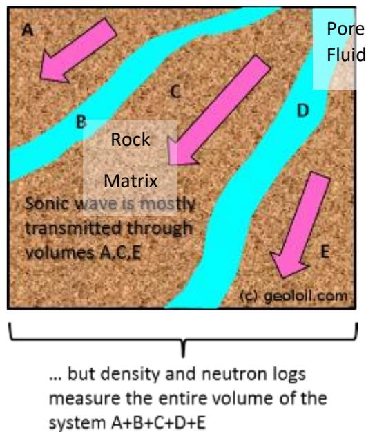
Figure 3. Illustration of how the sonic wave transmitted in the rock. The sonic wave will tend to ‘choose’ propagating in the dense medium such as through matrix where the transit time is faster. Therefore, it will cause the porosity estimated from the sonic to be lower than the ‘true’ porosity. (source: <https://geoloil.com/fracturePorosity.php>)
