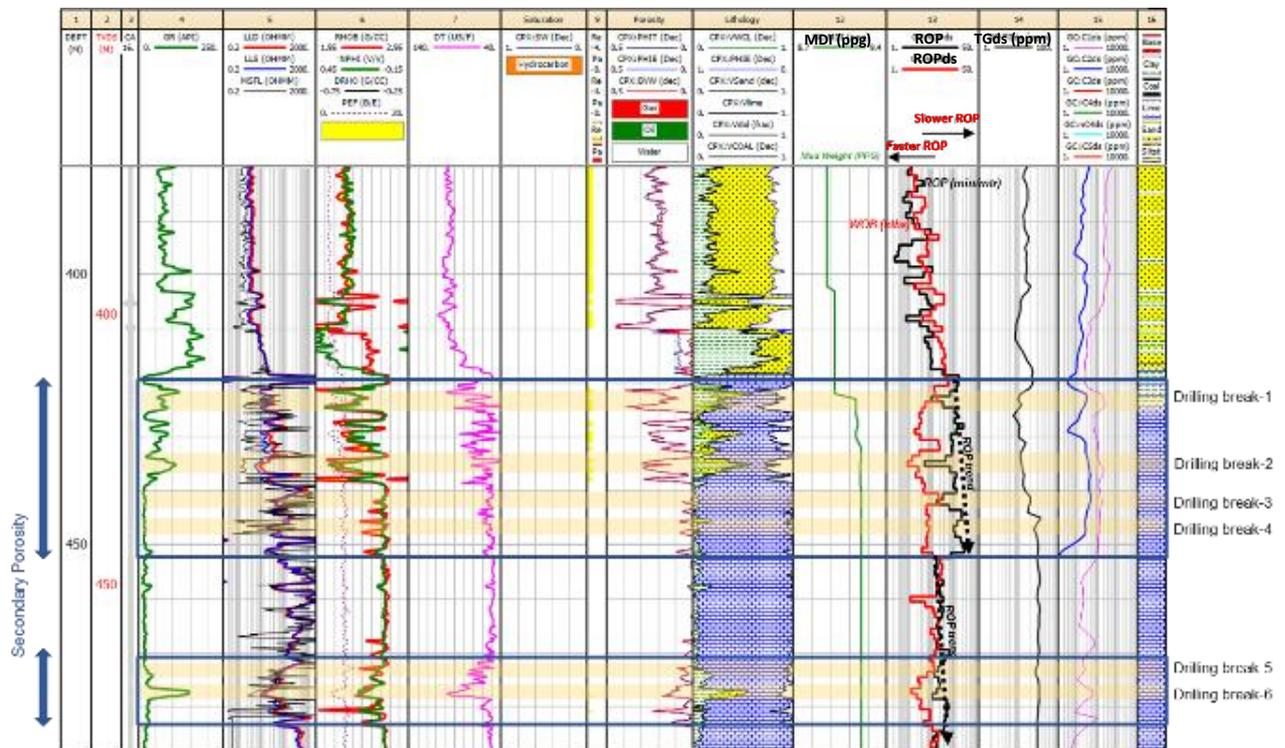
Figure 6. Drilling break events in carbonate basement of “X-1” well (highlighted in brown) as the proposed well testing interval in “X-1” well.
