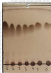
Figure 3. The Chromatogram of reaction for the 1 st until 6 th hour (s) Oleic acid and ( 1 st until 6 th ) Reaction time; Eluen n -hexsane:ethyl acetate (8:2)
