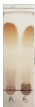
Figure 2. The Chromatogram of reaction for the 1 st hour (a) Oleic acid and (b) Crude reaction; Eluen n -hexsane:ethyl acetate (8:2)
