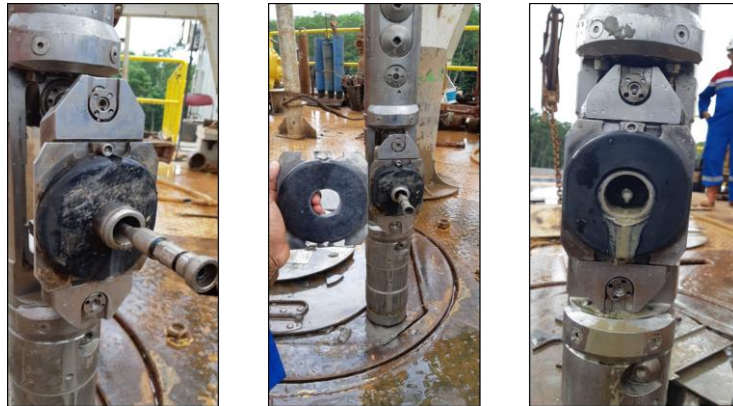
Figure 4. The Extra Large Probe Diameter which found error in reading (left) then replaced by the back up tools (middle and right).
