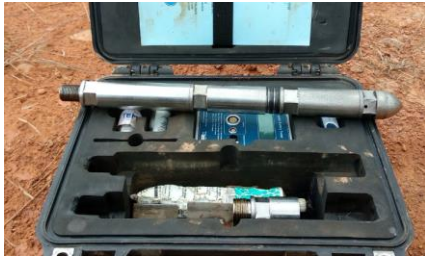
Figure 6-EMR as downhole pressure survey
