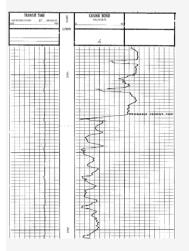
Based on the image of DRO-48 production profile, it shows that the gas from the ES layer has returned to production after the cement bond repair in 2016. This also affects its lifetime to extend.
