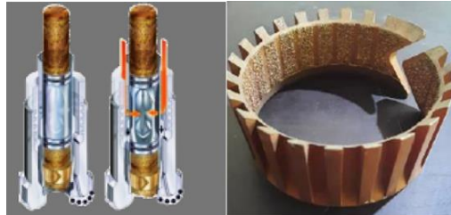
Figure A 2 (Left) Gripping Sleeve will collapse on soft formation, (right) secondary heavy duty spring catcher to hold hard formation
