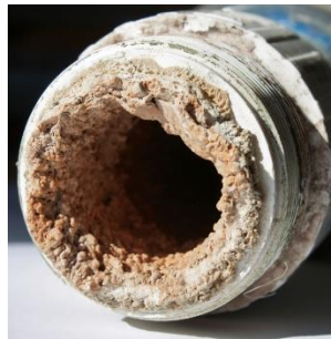
Figure 2. Scale issue in tubing
