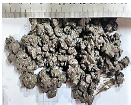
Figure 4. Cuttings observed on shakers
