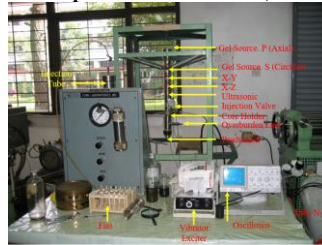
Figure 8. Vibroseis EOR laboratory equipment to stimulate the vibration of axial (longitudinal, P waves) and circular (transverses, S waves)
