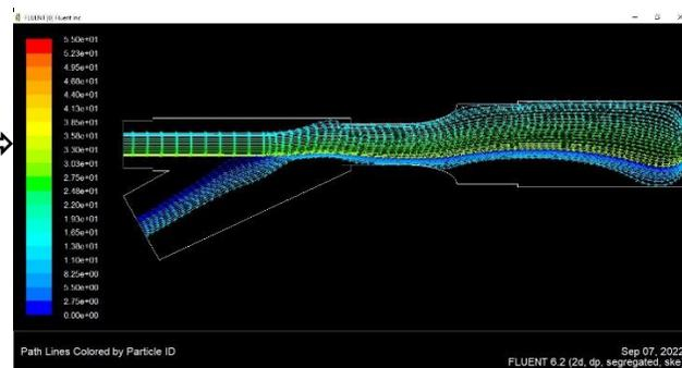
Figure 4. Y Type Ejector path lines result
