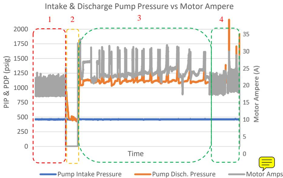
Figure 7. ESP parameter after ejector installation
