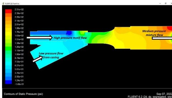
Figure 2. Y Type Ejector static pressure result
