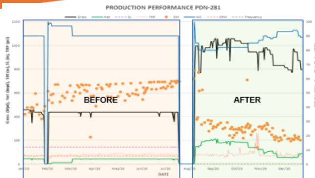
Figure 9 – The Comparison of PDN-281 Production Performance Before and After Convert Artificial Lift
