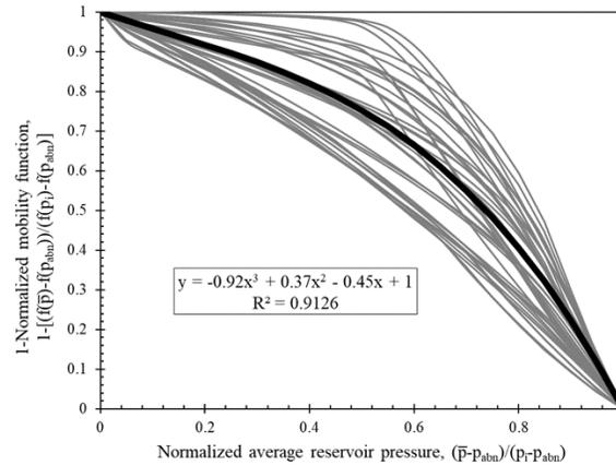
Figure 4. Generalized profile of normalized pressure vs normalized mobility function
