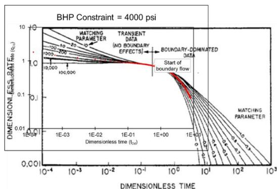
Figure B.1. Determination of the start of boundary-dominated flow using type curve from Fetkovich (1980)
