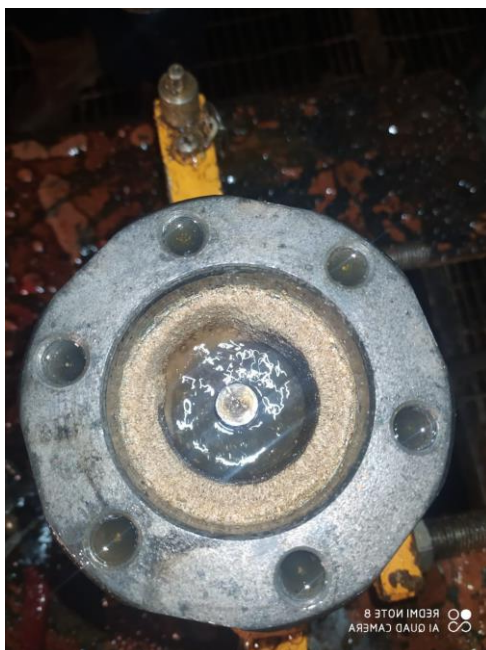
Figure 20 Scale deposition in pulled pumped Well GS-15
