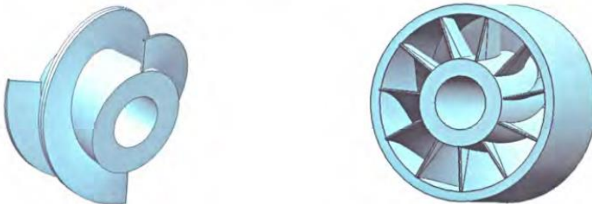
Figure 14 Axial type impeller and gas handling diffuser of an MPP (Peshcherenko et al, 2014)
