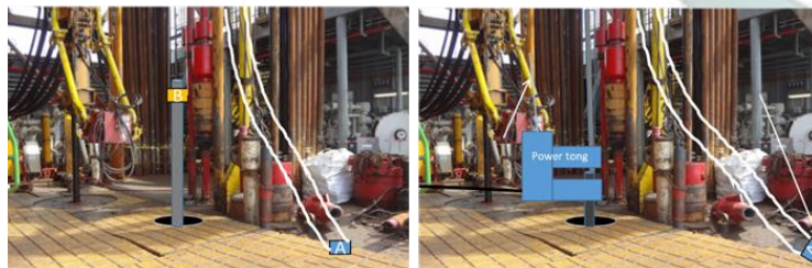
Figure 8. Makeup tubing 3-1/2" while drilling
