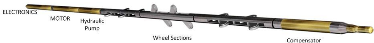
Figure 1 – Electric line Tractor
