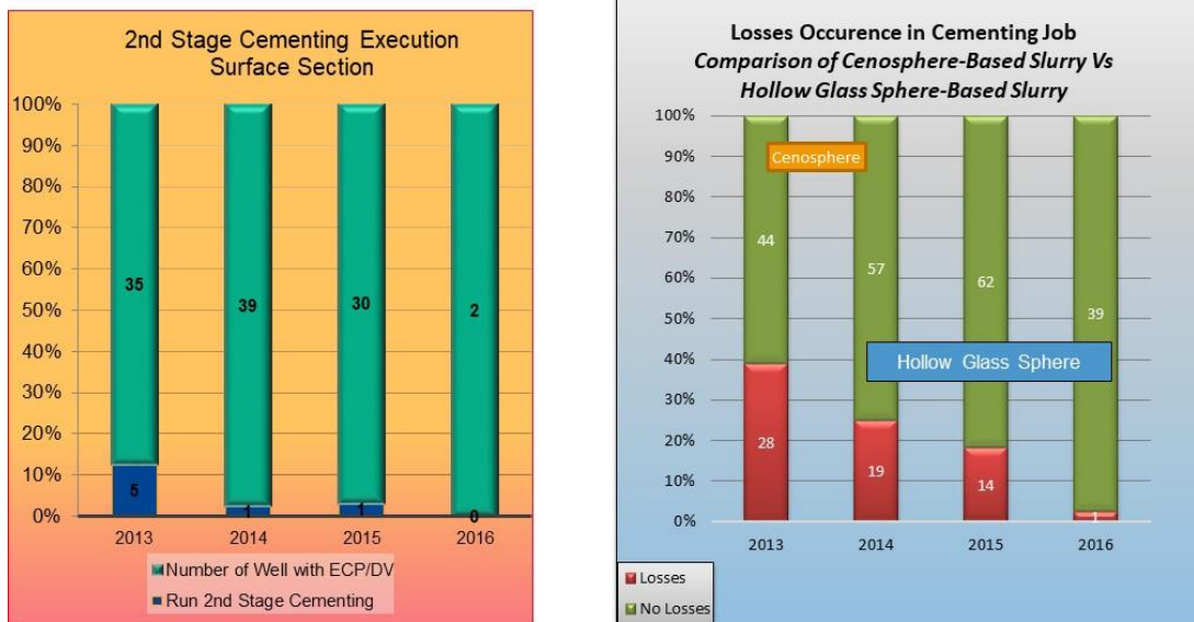
Figure 1.1 Statistic of loss circulation and second stage cement performed in the replacement of cenosphere to HGS
