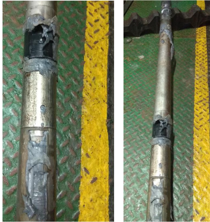
Figure 10. Recovered plug was found covered with Sealant residue
