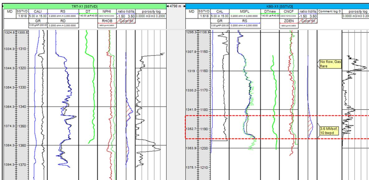
Figure 4. Type Log of Basement from Well TRT-X1 and KBS-X1
