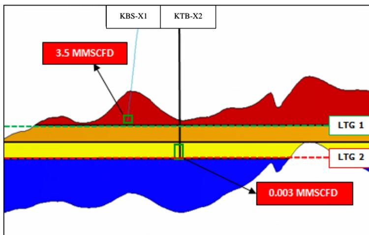
Figure 6. LTG Case 1 and Case 2 for Fractured Basement Volume Calculation
