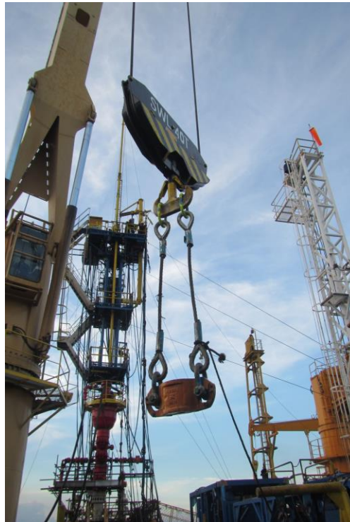
Figure 9 - Hoist System Using a Crane in the Main Barge
