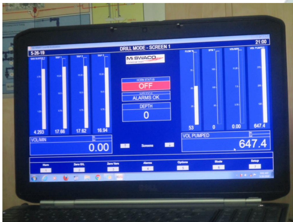
Figure 11 - Sensor Display on Trip Tank Connected to the Supervisor Room.
