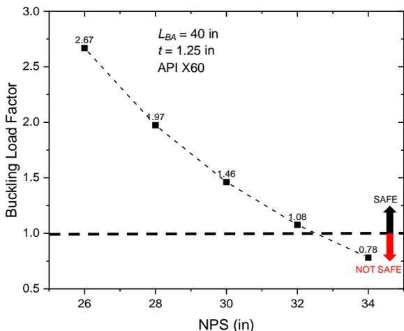
Fig. 7. Numerical simulation results: buckling load factor vs pipe diameter
