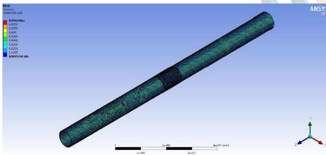
Figure 3. Solid model meshing
