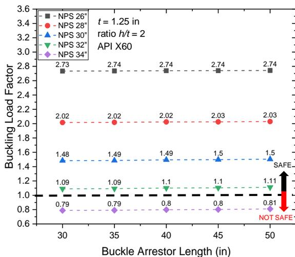
Fig. 5. Numerical simulation results: buckling load factor vs buckle arrestor length
