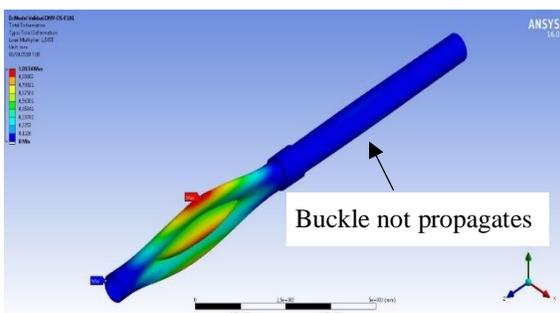
Fig. 9. Mode shape of pipe deformation NPS 28" when a ratio of buckle arrestor to pipe thickness is higher or equal to 3.0
