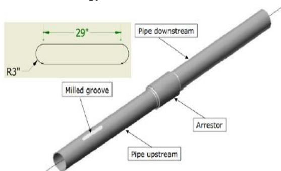
Fig. 1. Integral buckle arrestor configuration [1]
