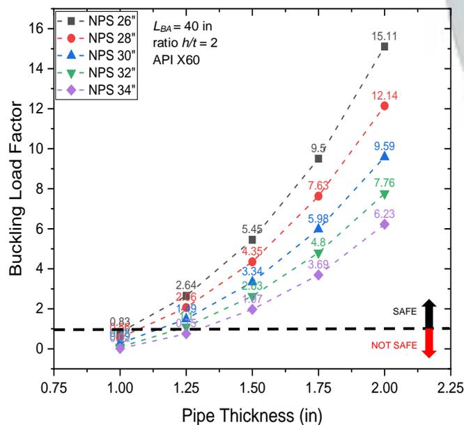
Fig. 4. Numerical simulation results: buckling load factor vs pipe thickness
