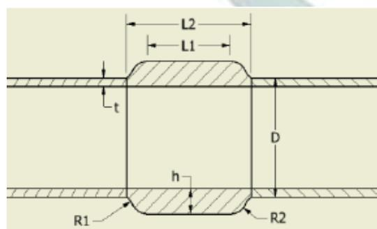
Fig. 2. Cross-section of integral buckle arrestor
