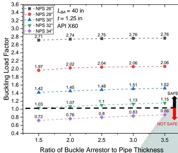
Fig. 6. Numerical simulation results: buckling load factor vs ratio of buckle arrestor to pipe thickness
