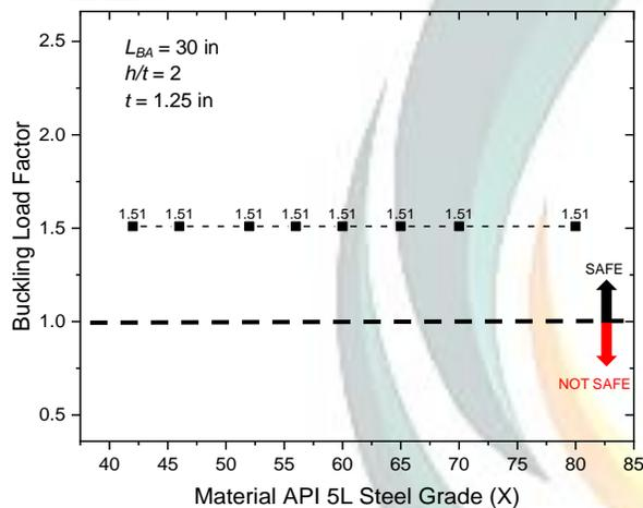
Fig. 8. Numerical simulation results: buckling load factor vs buckle arrestor material
