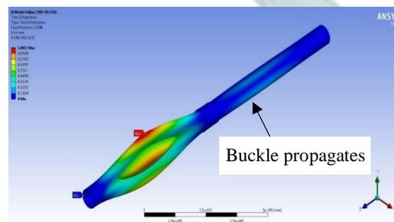
Fig. 10. Mode shape of pipe deformation NPS 28" when a ratio of buckle arrestor to pipe thickness is less than 3.0
