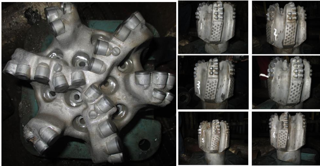
Figure 15. Dull Condition of Unique Hydraulics Bit First Trial
