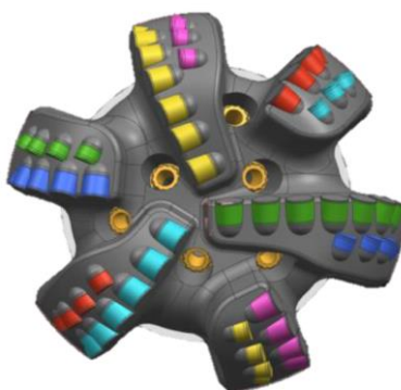
Figure 9. Efficient Backup Cutter Layout Cutting Structure
